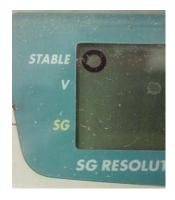
Figure 17: Circle indicates "Stable" weighing condition
