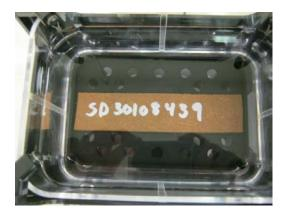
Figure 20: Specimen centered correctly on sensor weighing basket
