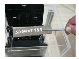
Figure 19: Using forceps to place specimen Gently on sensor weighing basket
