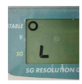
Figure 18: "L" shows weight is measured in ethanol
