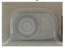
Figure 7: Correct position of air bubble within red circle of level indicator
